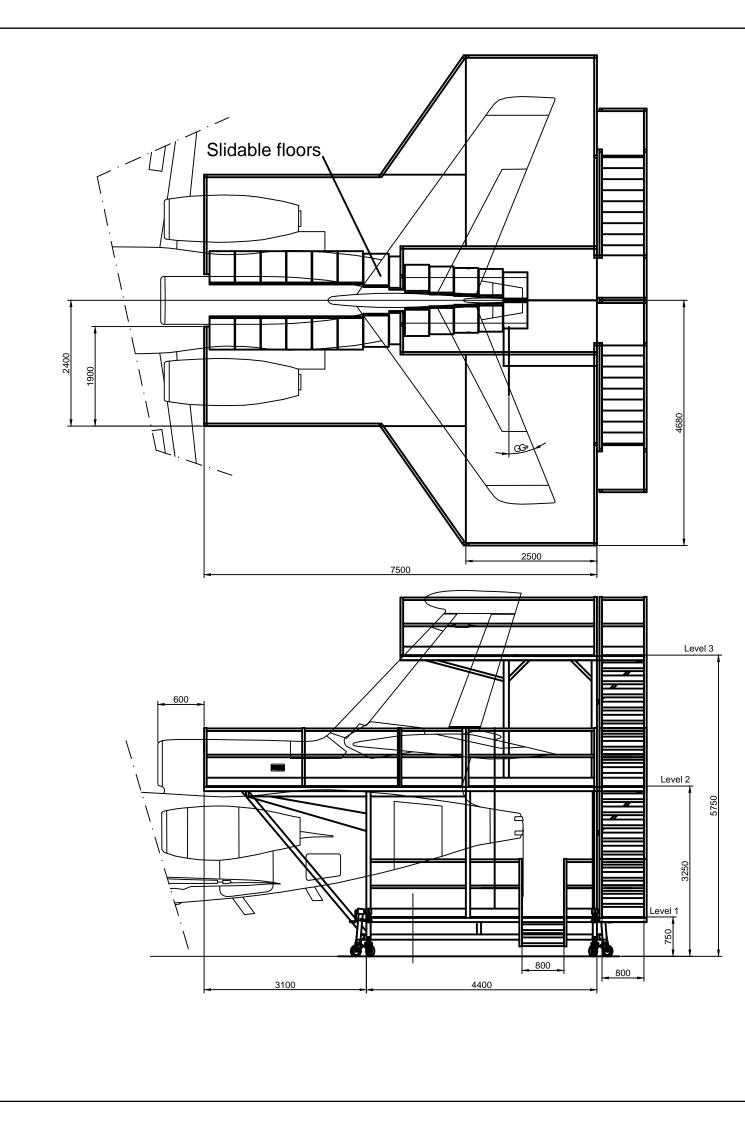
Tail Dock Falcon 50: -construction: aluminium -floors: checker plate -stairs: checker plate -wheels: max. load 1000 kg / double brake -height adjustment: 45 cm
